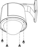
11. Make sure that all the devices are connected correctly to the camera and then check the functions of the camera. If there are no problems, affix the housing onto the wall mount using the three screws.
